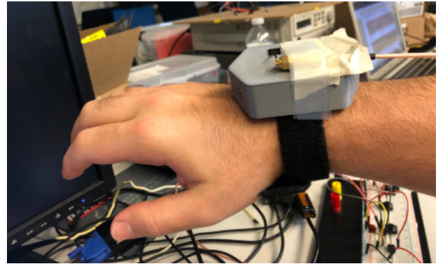
Fig. 4: The wearable device containing the required sensors.
